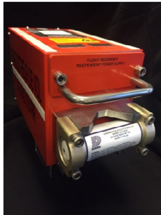
DK120/90 Dukane Seacom 90-day beacon, same form/fit as the original 30-day model
